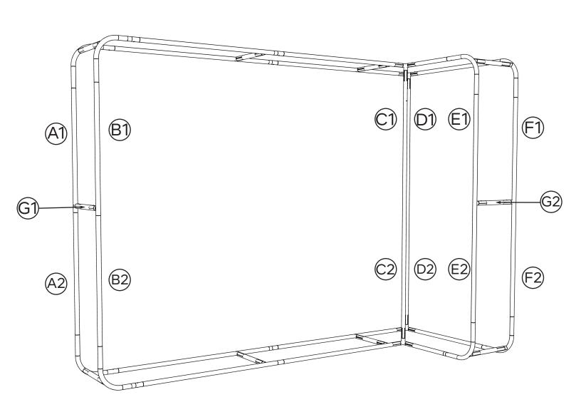
Press button & insert swaged end into receiving end of tubing
