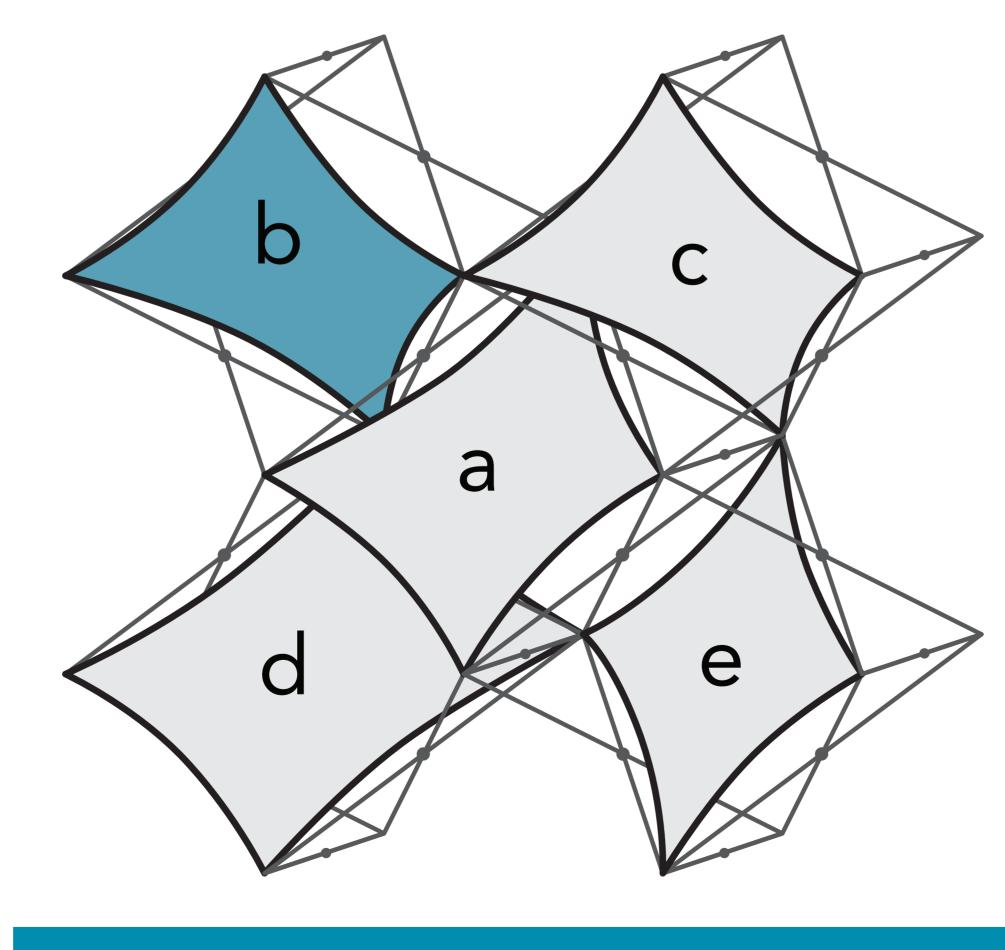
X-FACTOR: A term describing the result of tension at all corners and connection points of an Xpressions skin when placed on a frame. The artwork will be stretched with the least amount of distortion at the center of each quad, and the most distorti within the outer 3-5" of the skin. It is not a live area, as the image will be visible.
