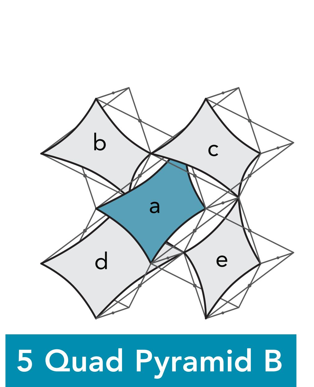
X-FACTOR: A term describing the result of tension at all corners and connection points of an Xpressions skin when placed on a frame. The artwork will be stretched with the least amount of distortion at the center of each quad, and the most distorti within the outer 3-5" of the skin. It is not a live area, as the image will be visible.
