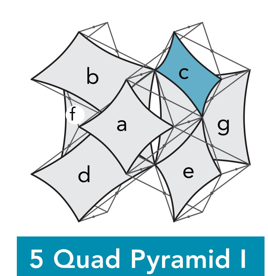
X-FACTOR: A term describing the result of tension at all corners and connection points of an Xpressions skin when placed on a frame. The artwork will be stretched with the least amount of distortion at the center of each quad, and the most distorti within the outer 3-5" of the skin. It is not a live area, as the image will be visible.
