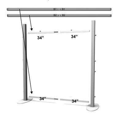
**Step 4.** Place canopy on columns. Tighten column top CBX clamps using Red/Black handle 5mm hex wrench.
