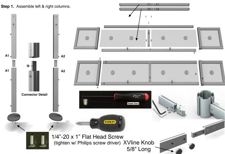
**Step 2.** Join 2-piece graphic bars together; attach top cross bar to column; align with arrow.
