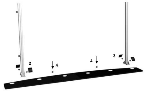
Steps 5&6. Attach left and right lower columns to feet using 2 short knobs per column. Install gusset caps.
