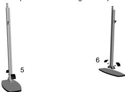
**Steps 7,8**. Tip canopy and legs down; attach left and right lower columns to upper columns using 2 **short** thumb knobs per column.
