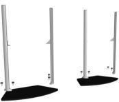
**Step 12**. Attach counters to backwall from underneath using one **long** knob for each counter. Attach shelf using 3 **long** knobs per shelf.
