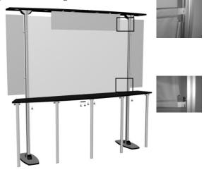
Step 13. Install 4 front panels and 2 end panels.
