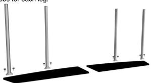
**Step 12**. Attach counters to backwall from underneath using one **long** knob for each counter. Attach center leg using 2 **long** knobs. Join back of counter using plastic joining plate and 2 **long** knobs.
