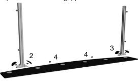
**Steps 5,6**. Attach left and right lower columns to feet using 2 **short** knobs per column. Install gusset caps.
