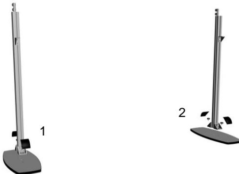
**Step 3.** Attach counter legs to counters using 2 **long** knobs per leg.
