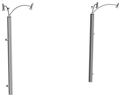
**Steps 6&7.** Attach left and right upper columns to lower columns using 2 **short** knobs per column.
