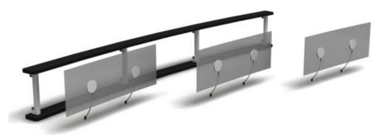
Steps 5&6. Attach left and right lower columns to feet using 2 short thumb knobs per column. Install gusset caps.
