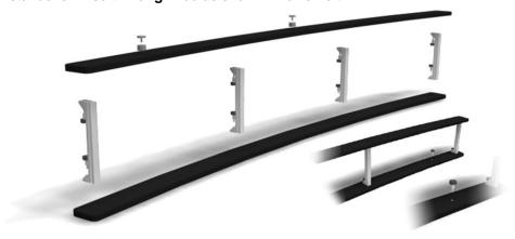
Step 4. Insert plex w/ pre-installed puck lights. Attach one 3-way power splitter to left 3 lights and one to right 3 lights.
