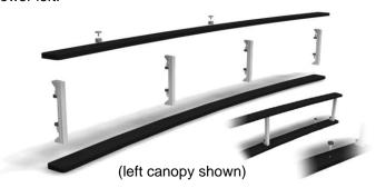
**Steps 7&8**. Attach left and right lower columns to upper columns using 2 **short** thumb knobs.
