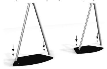
Step 13. Attach counters to backwall using one long knob per counter. Attach legs to bases using 1 long knob per leg.
