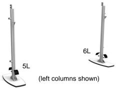
**Step 10**. Slide canopy supports onto columns and tighten **short** knobs. Place canopy onto supports.
