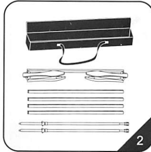
2. The case should contain a base unit, a telescopic pole and 4 snap bars.
